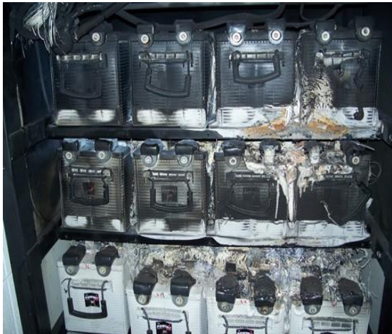
Container Destruction due to Thermal Runaway
