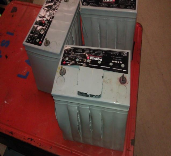
Container Destruction due to Thermal Runaway
