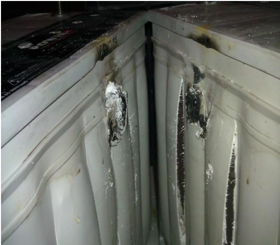
Explosion due to Thermal Runaway
