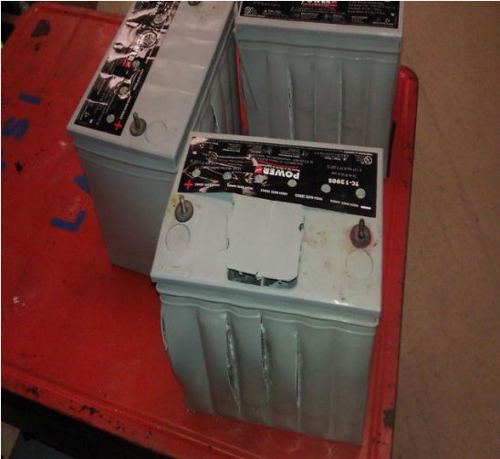
Container Destruction due to Thermal Runaway
